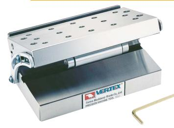
Design by the principles of SINE, angle grinding can be done well. High precision of parallelism within 0.002 mm and squareness within 0.005 mm. Setup and dressing time reduced to a bare minimum due to simplicity.(ANGLE 0° - 46°)
